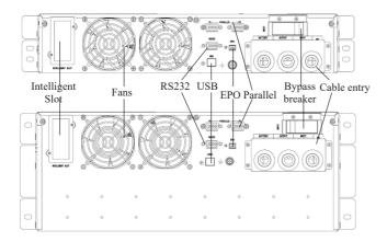
As shown in Fig 1-2, the rear panel provides the following compoentes and function:
